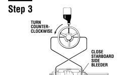
• Hold the cylinder body to prevent the rod from moving and turn the wheel counter-clockwise until a steady stream of air free fluid flows from the bleeder nipple.
