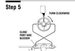
• Hold the cylinder body to prevent the rod from moving a turn the wheel clockwise until a steady stream of air free fluid flows from the bleeder nipple.
