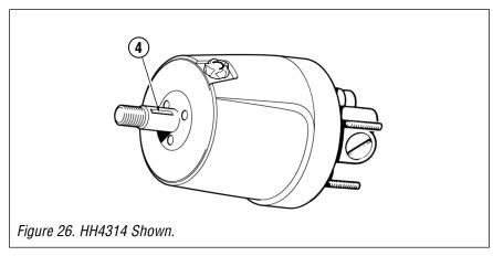
**4.** Remove steering wheel; clean off helm pump shaft; re-grease using a good quality marine grease.
