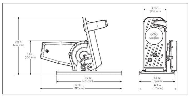
**3** Front (Bow) Mount Engine Control Dimensions
