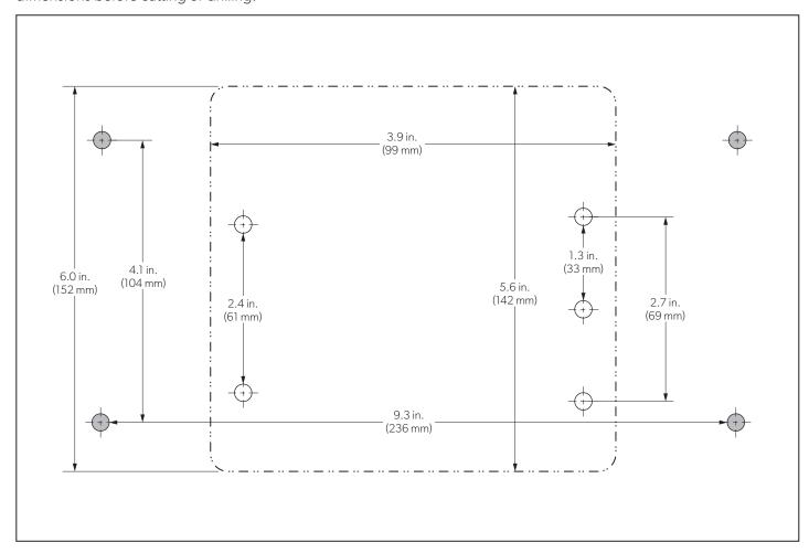
Hole location for mounting the engine control directly to the boat deck
