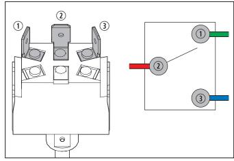
2 Switch Wiring Diagram
