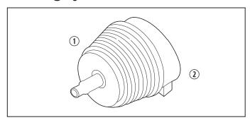
13 Performance Tilt Steering System Boot and Bezel
