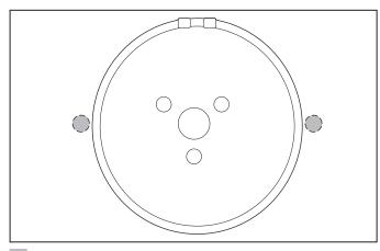
**20** Hydraulic Steering System Wire Passage—Option 1 Holes
