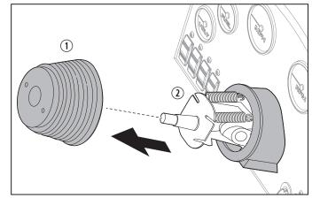
15 Performance Tilt Steering System Holes in Mounting Flange(1) Boot(2) Tilt Mechanism
