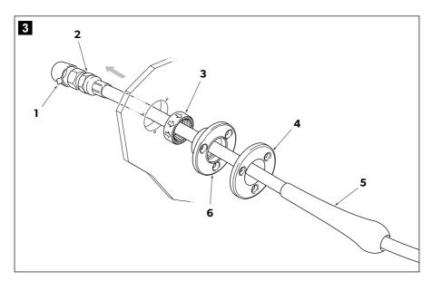
With the dust caps still installed, feed the hoses from the outside of the boat through the newly drilled holes, inside along the gunwale or rigging tube to the desired steering system component. The mounting plates, knurled nuts and bend restrictors must remain outside the boat hull.
