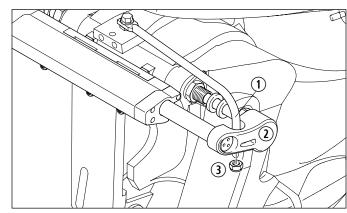
12 Securing the Engine Link Arm
